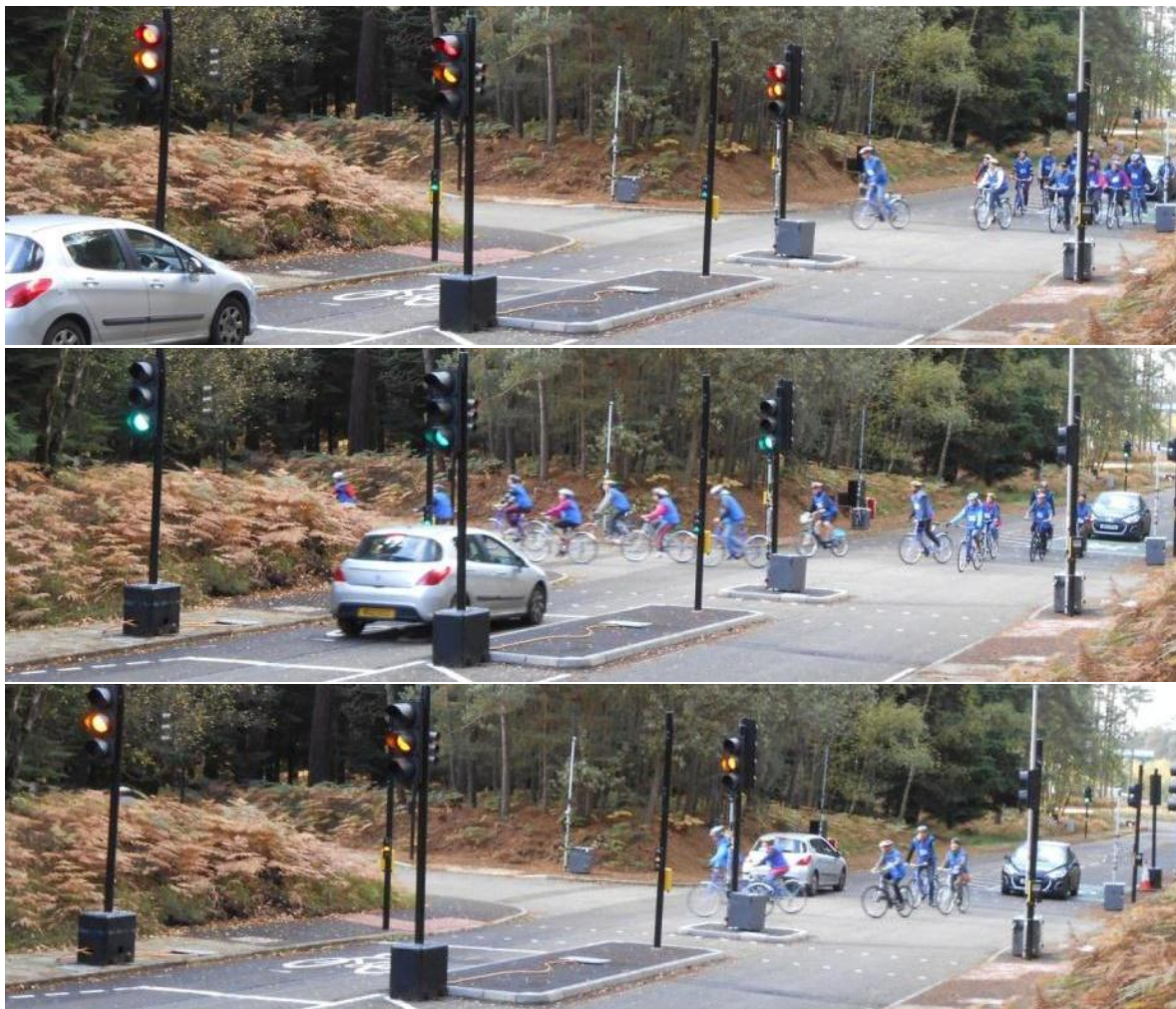
Figure 29 – Cycle trial: example of cyclists turning in front of oncoming car
