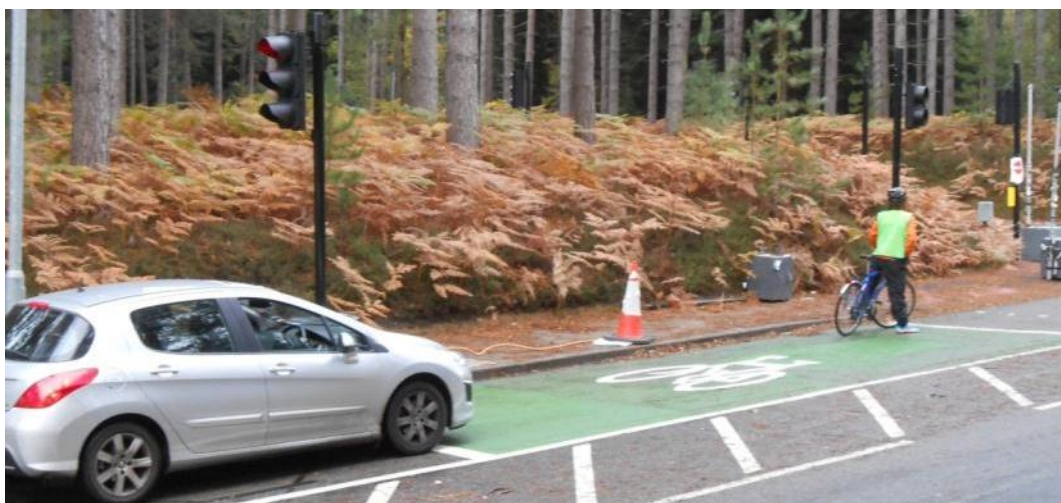
Figure 37 – Car trial: example of a car stopped past the first stop line
