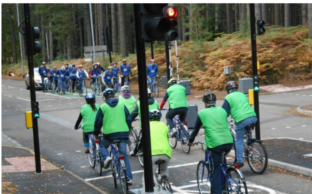
Figure 22 – Cycle trial: photo of groups of cyclists moving off when the LLCS were green and the main signals were red
