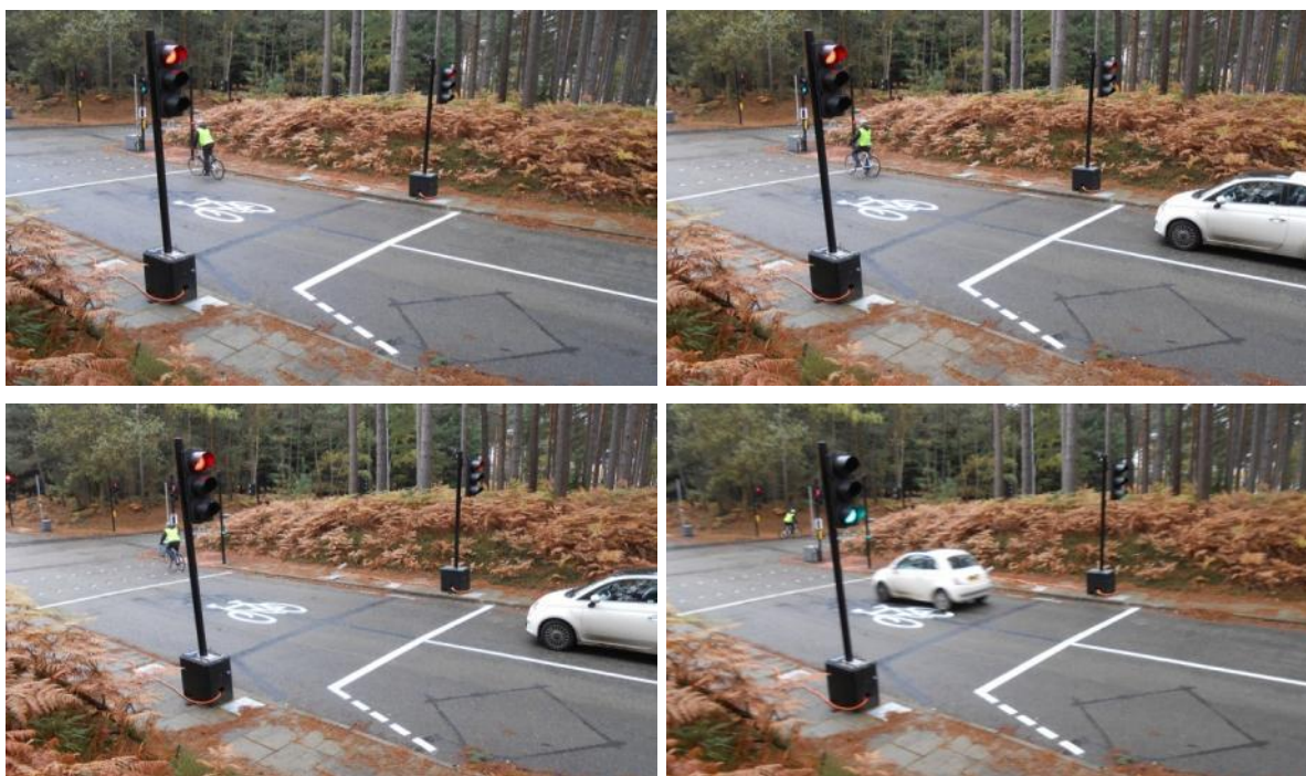
Figure 44 – Car trial: example of a car entering the junction after the cyclist
